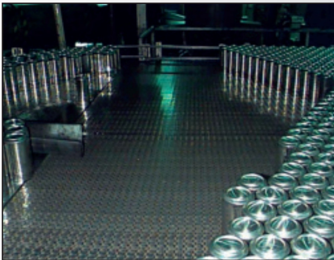
CAN WASHER DISCHARGE WITH 5936 BELT
