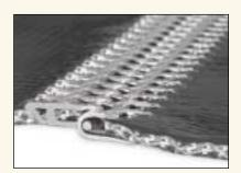
Alligator® Lacing teeth enter parallel to the length of the belt and embed clear through the belt carcass. The design of the teeth ensures that once they are driven into the belt, the vital longitudinal carcass fibers are not severed.
