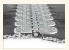
Staples penetrate between carcass fibers without severing them. Staples are hammer-driven through the belt and then clinched crosswise to prevent belt tension from pulling against – and unclinching – the staples.
