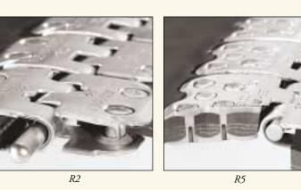
The SR<sup>™</sup> (Self-Setting Rivet) Fastener utilizes staggered pattern, multiple rivet attachments that pass between carcass fibers without severing them. The specially shaped head of each pilot nail works in conjunction with the installation tool anvil plate to set the rivets. The same hammer blows that set the rivets also compress the fastener plates into the belt covers. This provides maximum holding ability and distributes splice tension evenly across the width of the belt.
