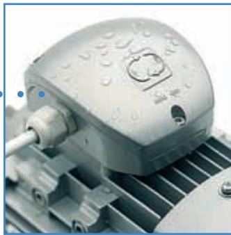
Aiming the maximum protection, the motors are equipped with important details like the pull-resistant cable press and the combination of bearings with two shields each with rubber seal rings
