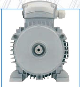
From size 56 to size 132, feet are detachable, and can be fixed on 3 sides of the housing, thus permitting the terminal box to be positioned up, right or left.
