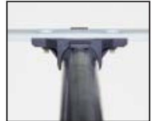
**BOLT-ON VERSION** - When roller removal is desired, the **EZ Roller Retrofit Bolt-On Component** is recommended. Sturdy 5 foot sections are pre-assembled to save labor, and bolt into existing roller 7/16" (11 mm) hex holes (only eight bolts per section required). A chevron wearstrip pattern increases belt life.
